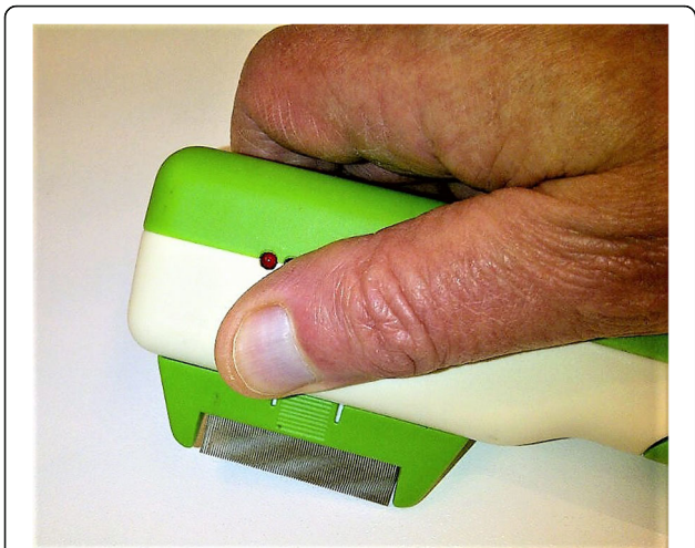
Fig. 4 Hand position taken up by investigators, close to the tooth unit, in order to retain a firm grip whilst combing. Moving the hand to this position largely eliminated the angle of the combing head, which had previously been shown to improve louse egg removal. Consequently, this would have resulted in some of the extra combing efficiency delivered through the ultrasound actuation being lost in practice
